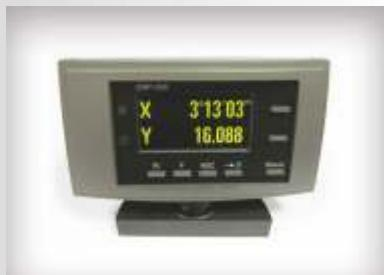
Compact DRO for 2 axes. It can be used with angular and linear encoders.
