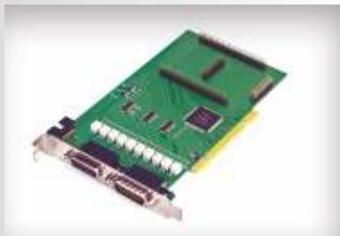
Can be embedded inside of a PC or serve as a separate block with connection to RS-232 or USB ports. Works also with ISA and PCI buses. Up to 4 encoders can be connected at the same time. SKBIS offer interfaces for absolute and incremental encoders.
